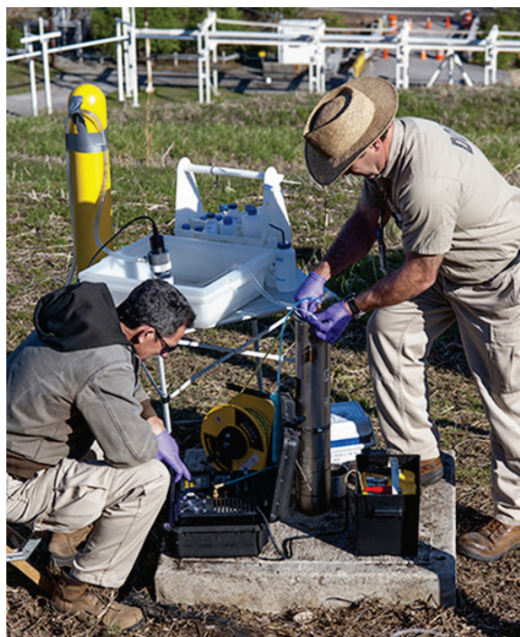
Fig. 4.38. Groundwater monitoring well sampling at Y-12. [Source: Kathryn Fahey, Y-12 photographer.]
